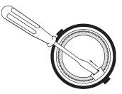
The adapter can be remove simply by pressing the adapter clip on the underside of the actuator
